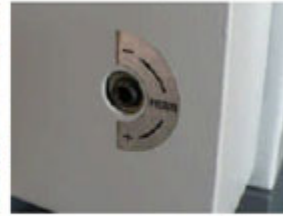
Electric edge folder Adjustment for pressure of edge folder
