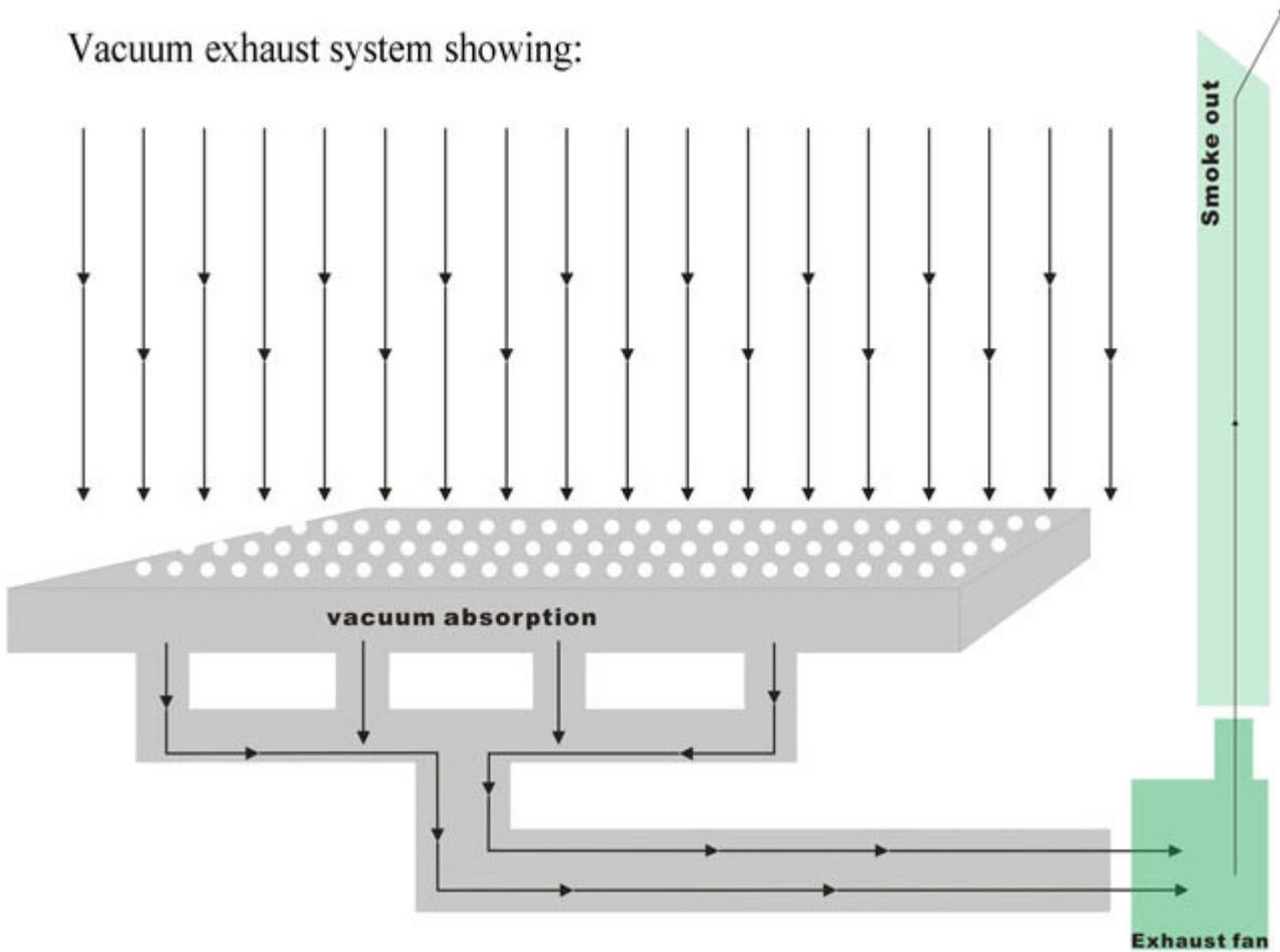
The vacuum absorption working table has the largest strength for absorb the material close to the table and to be flatted; exhaust system for taking away the smoke with pollution circumstance.
